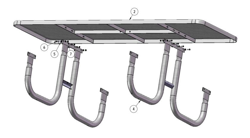
Attach the 8' Expanded Top to the 238 Frames using specified hardware.
