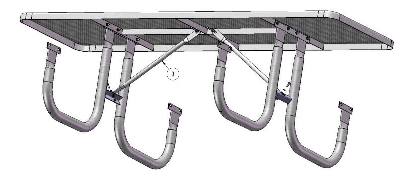
Attach the 29-7/8" Braces to the 8' Expanded Top and the 238 Frames as shown using specified hardware.
