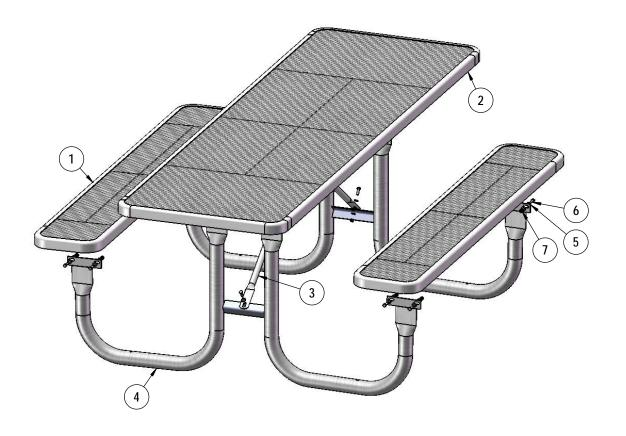
Optional Surface Mount Hardware: 5/16" x 5-1/2" Concrete Expansion Anchor Bolts (Not Included)
