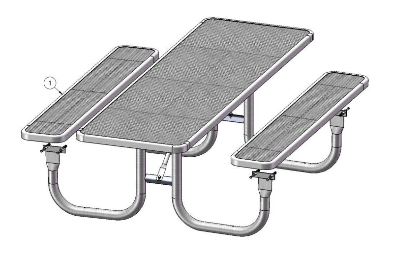
Attach the 6' Expanded Seats to the 238 Frames using specified hardware.
